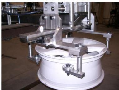
A variety of alloy rims with different dimensions (17" – 22" inch diameter) had to be accommodated at a production rate of 300 rims / hour.
