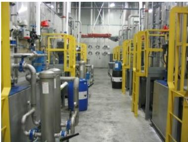
The line prepares the rim's alloy metal surface for liquid and powder painting using a 15 stage pre-treatment system, supported by 10 chemical
