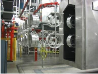
The line used three separate material handling conveying systems, one overhead and two in-floor conveyors.
