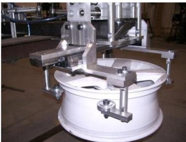
A variety of alloy rims with different dimensions (17" – 22" inch diameter) had to be accommodated at a production rate of 300 rims/hour.
